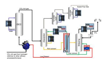
Designing the process to maximize the return temperature of the cooling water from the coolers and condensers reduces cooling water consumption by at least 50%. Alfa Laval plate heat exchangers can do this very cost effectively, in a single heat exchanger, while requiring minimal plot space.
