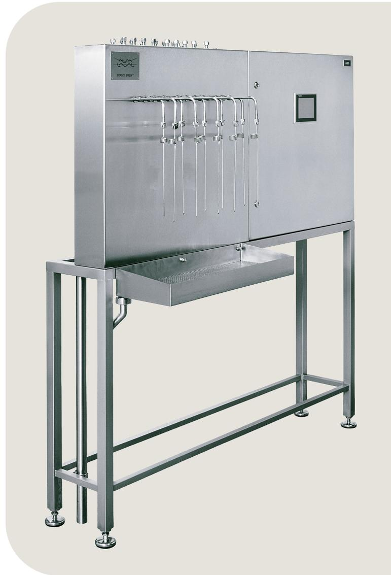
The sampling panel is connected via pipes of Ø10 mm to the pneumatic sample valves on the tanks. The connections can either be stainless steel pipes or Teflon hoses, with or without insulation, depending on local conditions.
